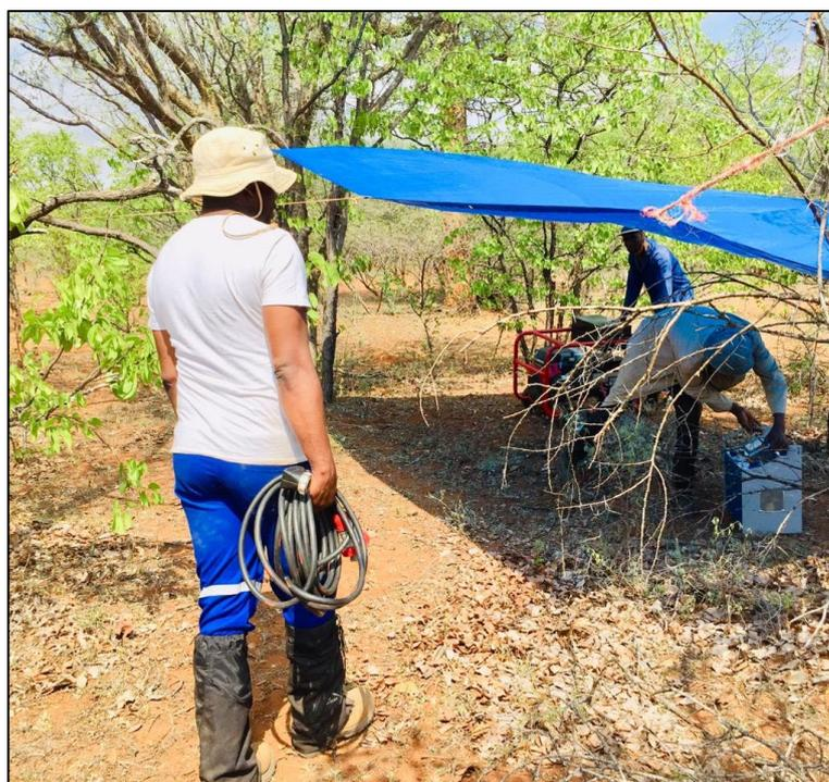
**Figure 2:** Field crew in Botswana undertaking Gradient Array IP surveying at the Airstrip Prospect.
