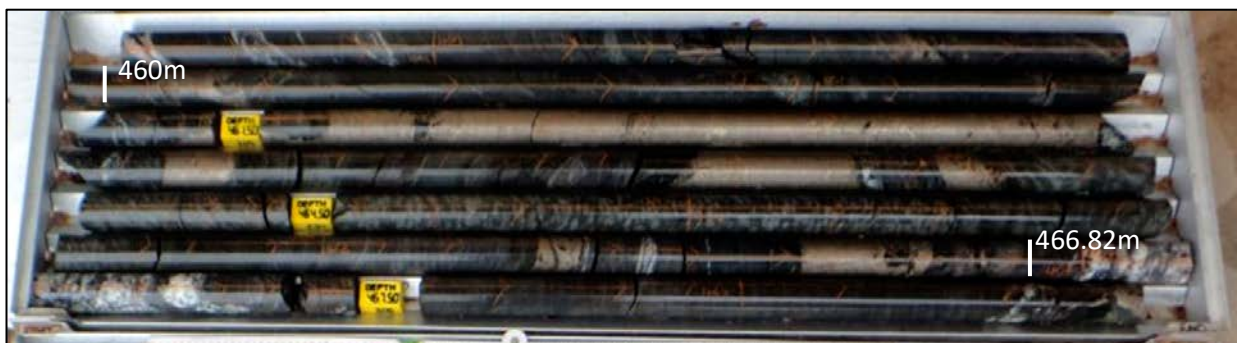
Figure 2: Photograph of sulphide intersection with massive, and semi-massive pyrrhotite from MARD0094
